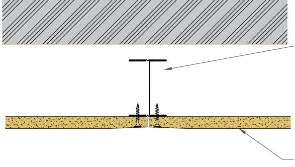
SPEEDLINE 60mm 'I' Studs at 600mm Ctrs
